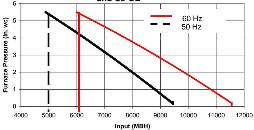
The Capacity Charts are based upon 2,000 foot elevation, 80 degree F combustion air temperature, firing with 15% excess air (3% O<sub>2</sub>) and standard diffuser blade settings. If job conditions vary from above conditions, capacity rates may vary.
