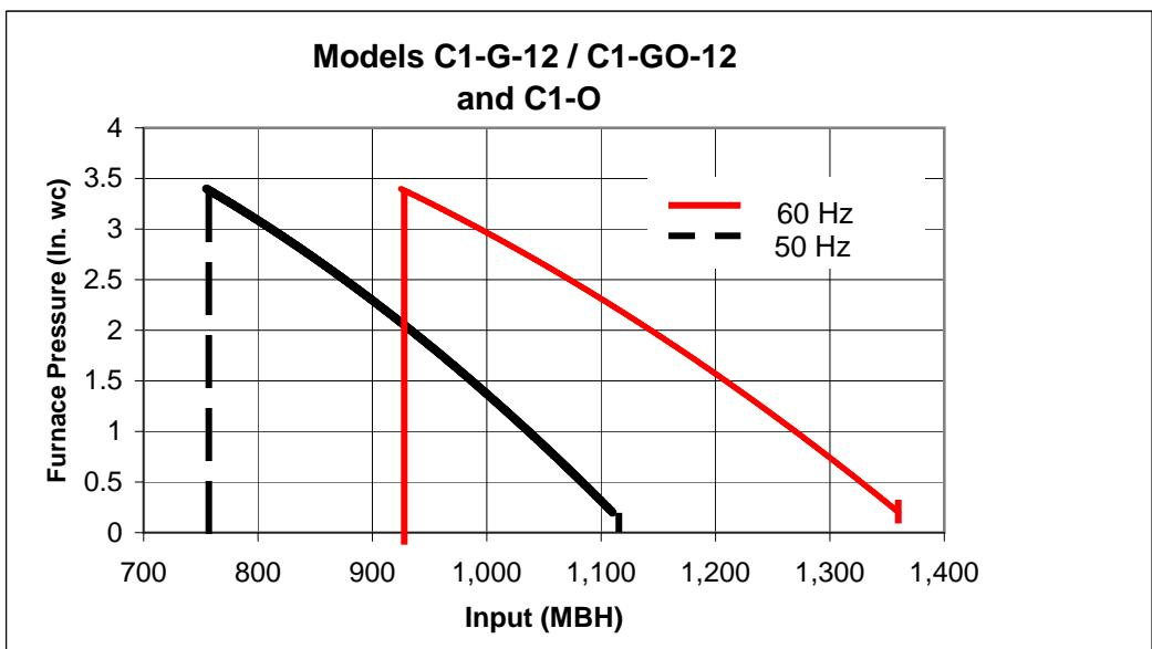
The Capacity Charts are based upon 2,000 foot elevation, 80 degree F combustion air temperature, firing with 15% excess air (3% O<sub>2</sub>) and standard diffuser blade settings. If job conditions vary from above conditions, capacity rates may vary.
