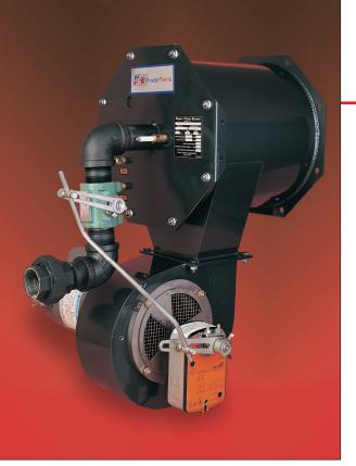
Model FDM-modulating pie shaped dampers allow close control of air/fuel ratios over a 20:1 turndown for special gas fired air handling applications.
